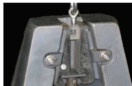
Fig. 5. Sample placed in the Instron universal testing machine for the pull-out test.
