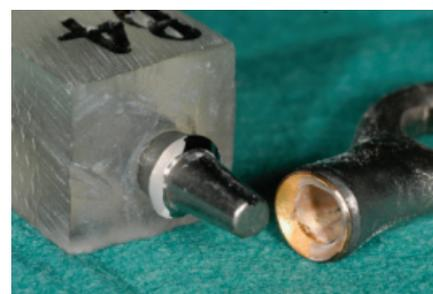
Fig. 6. Separation always occurred at the abutment–galvanic cap interface.
